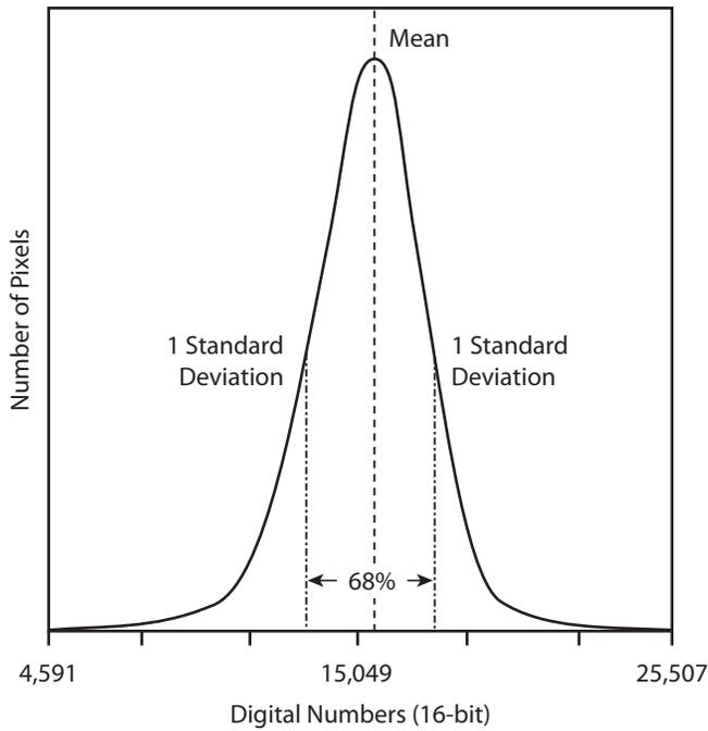
**FIGURE 9-3** Landsat OLI band 6 (SWIR1) input histogram with a mean DN of 15,049.
